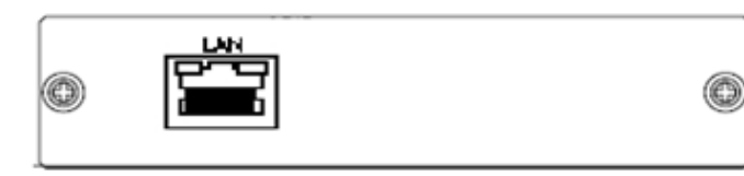
Figure 6: 44M04 LAN Connection
